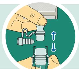
Step 2: To remove, pull out Connector with one hand while holding base of tap with the other hand.
