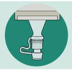
Make sure soft, ribbed cork is securely pushed into the bottom of the drainage tap.
