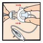
Connect the connector needle with the coupling housing.
