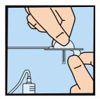
Prime the tubine according to pump manufacturer's instructions for use and remove the adhesive backing paper.
