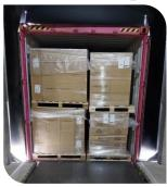
Convatec has adopted double stacking of pallets where feasible to enhance transport efficiency and reduce emissions. Left image (before) shows 53% space usage; right image (after) shows 90% space utilisation.
